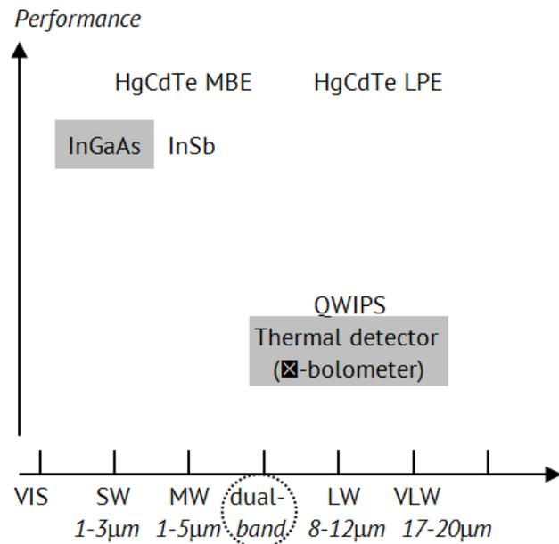
**Figure 4.**  $\text{HgCdTe}$  detectors grown by MBE and LPE deliver better object identification capability than the detectors, such as  $\otimes$ -bolometers and those based on  $\text{InGaAs}$  and  $\text{InSb}$   = uncooled; all other: cooled (after [7]).
