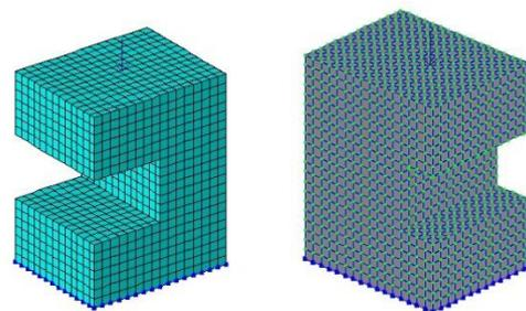
**Figure 6.** Finite Element Model of a Damaged Column.
