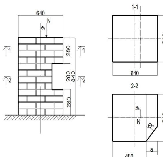
Figure 2. Diagram of simulation of damaged sample-pillar.
