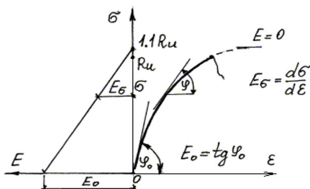
Figure 3. The deformation pattern of the masonry.
