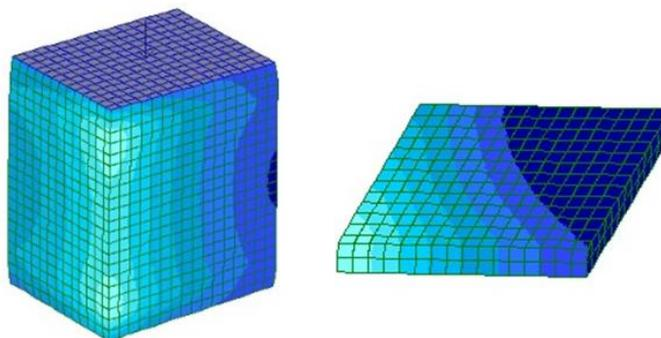
Figure 8. Isolation stresses in the C -1-1-1 column.
