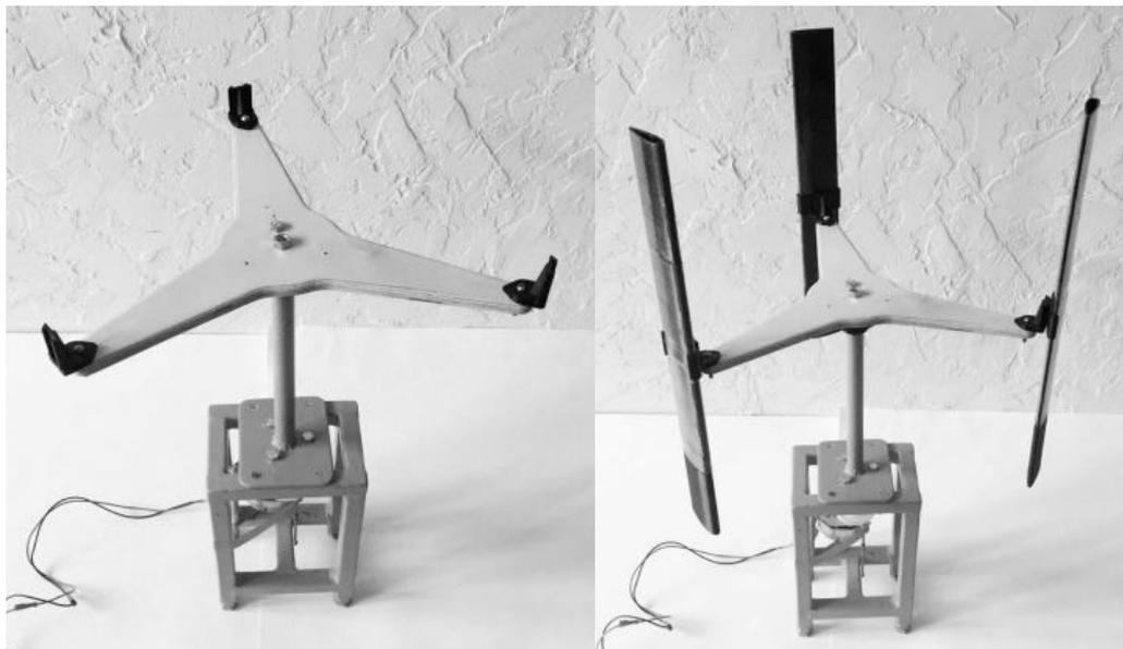
**Figure 4.** Experimental VAWT that allows changing different set of blades.
