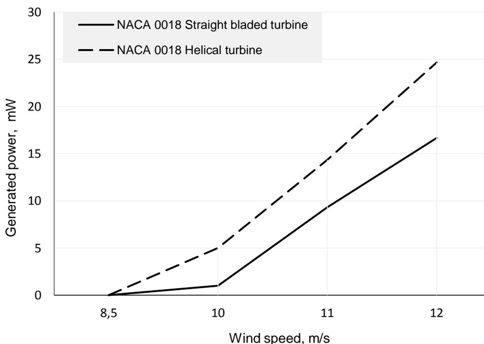
**Figure 6.** The performance of straight bladed and helical turbines based on NACA 0018 airfoil.
