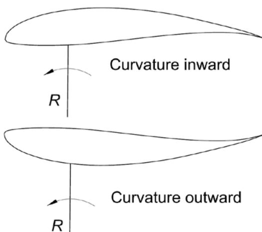
**Figure 7.** Airfoil curvature (camber) oriented radially inward and outward.
