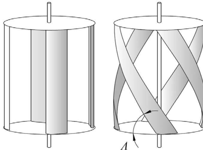
**Figure 1.** Straight and helically bladed turbines.
