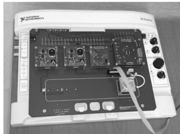
Figure 5. Data acquisition system NI Elvis II RElab.
