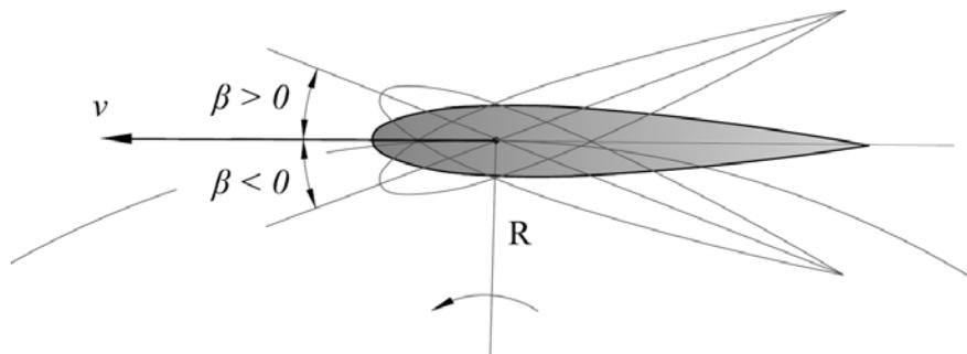
**Figure 3.** Pitch angle of the rotor's blade.
