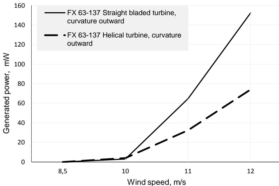
**Figure 8.** The performance of straight bladed and helical turbines based on FX 63-137 airfoil.
