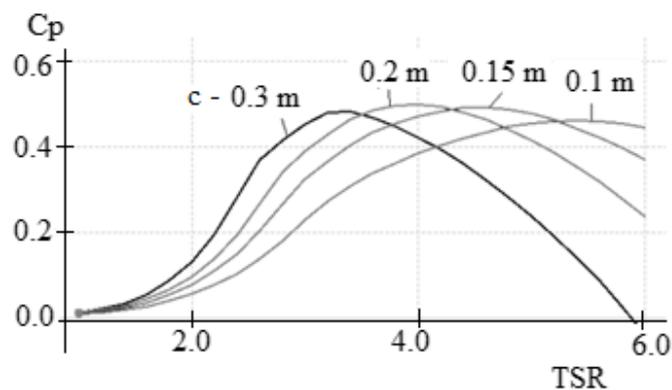
**Figure 2.** Power coefficient dependence on chord length.
