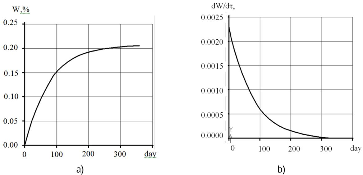
**Figure 1.** The water absorption curves (a) and the absorption rate (b) for the central composition ( $x_i = 0, i = 1-5$ )
