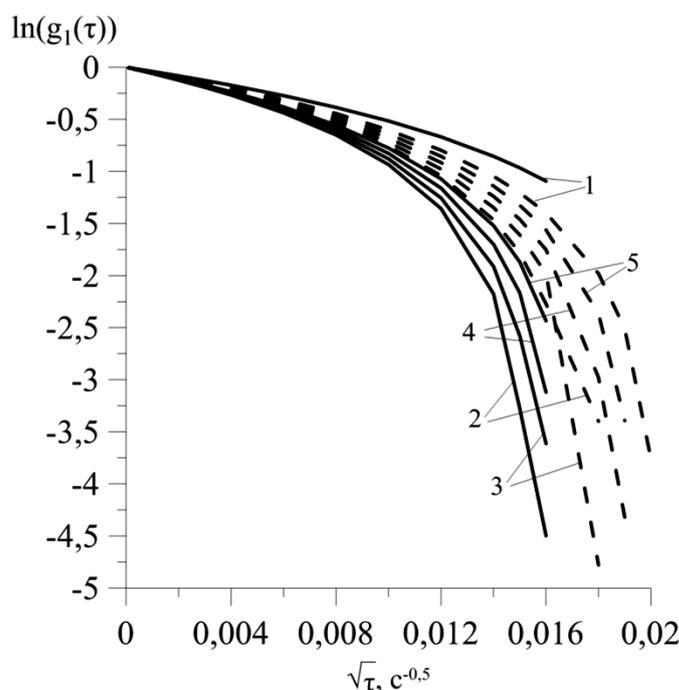
**Figure 4.** Typical autocorrelation functions  $g_1(\tau)$  of field fluctuations under conditions of different dynamics of blood flow in the experiment with compression of the brachial artery calculated in the MathCad system, 200  $\mu\text{m}$  - solid curves, 100  $\mu\text{m}$  - dashed curves
