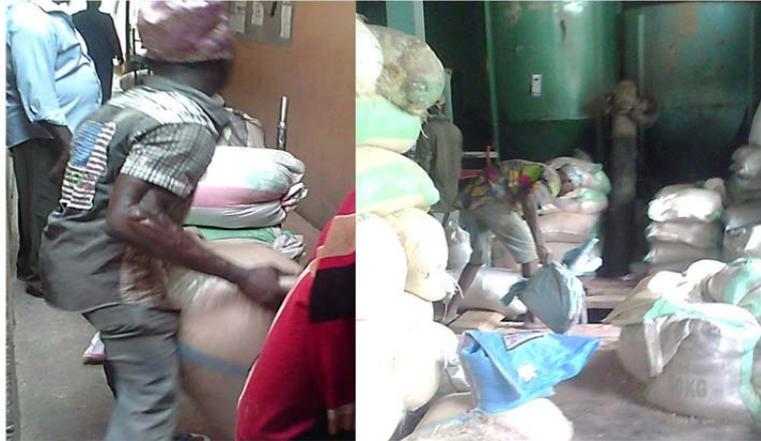
**Figure 7.** Manual material handling operation; loading hand truck (left), conveying materials during milling (right).
