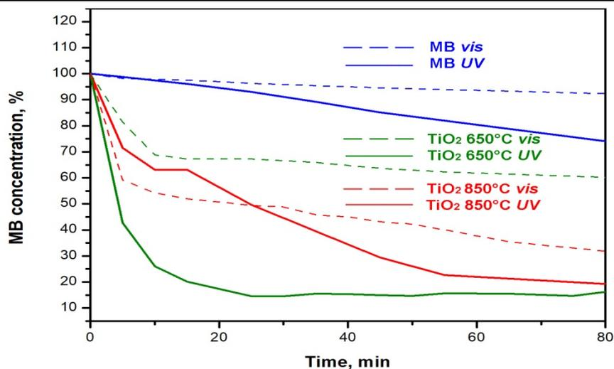
**Figure 4.** MB concentration decay in time in presence of 20 mg of TiO<sub>2</sub> nanotubes.
