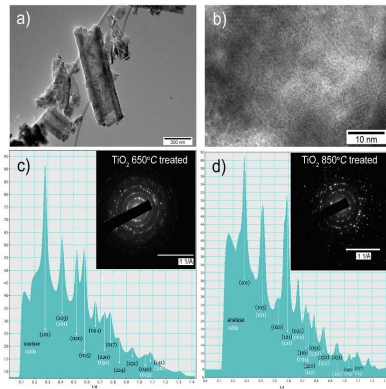
**Figure 2.** TEM analysis of TiO<sub>2</sub> nanotubes: (a) an overview image of nanotubes; (b) high resolution image of nanotube wall; selected area electron diffractogram and rotational average diagram of TiO<sub>2</sub> nanotubes treated at (c) 650 °C, and (d) 850 °C.
