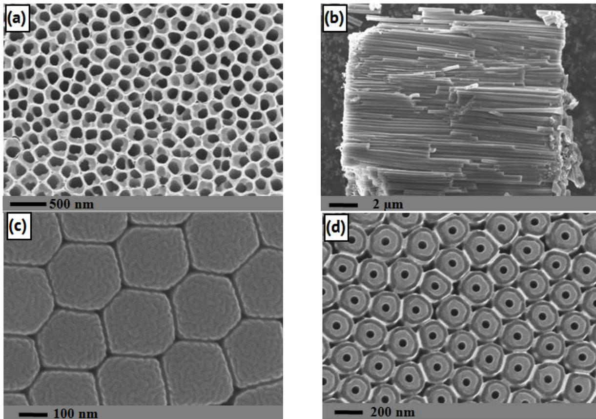
**Figure 1.** SEM images of TiO<sub>2</sub> membrane: (a) top part, (b) side view, (c) bottom part before dry etching step, (d) bottom part after dry etching showing opened nanotubes.
