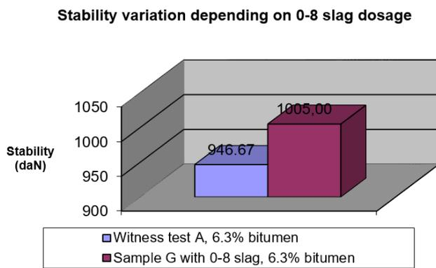
**Figure 1.** Comparison between Marshall stability determined on control and 0-8 slag samples.
