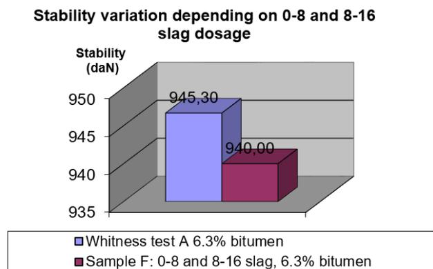
**Figure 4.** Comparison between Marshall stability obtained on control and 0-8+8-16 slag samples.
