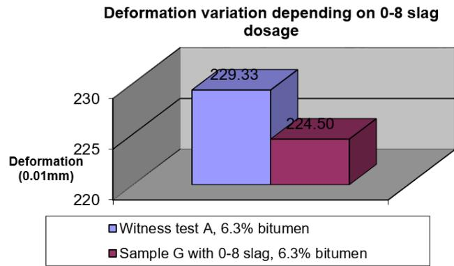
**Figure 2.** Comparison between the flow index determined on control and 0-8 slag samples.
