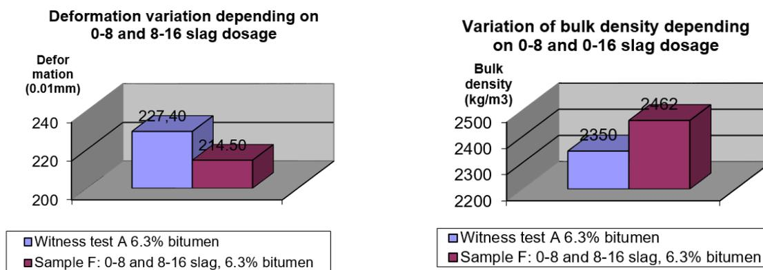
**Figure 5.** Comparison between the flow index determined on control and 0-8+8-16 slag samples.
