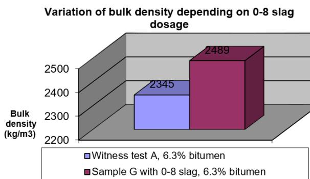
**Figure 3.** Comparison between bulk density determined on control and 0-8 slag samples.
