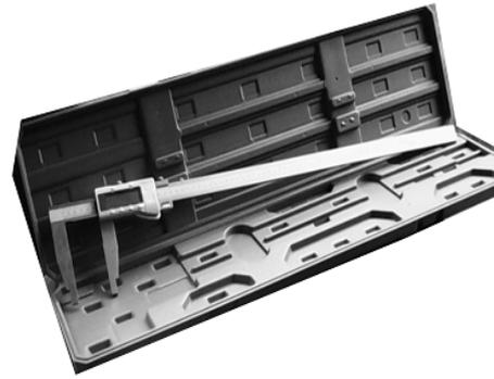
**Figure 2.** Digital Vernier caliper (600mm).
