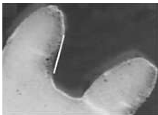
Figure 24. Reduction of the thickness of the polymeric tooth due to scraping of the opposite steel wheel, [35].
