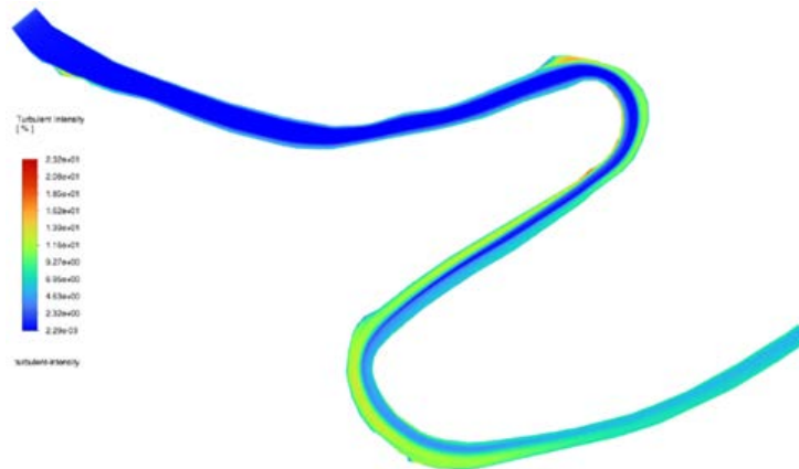
Figure 2. Turbulence intensity (%) on the 2D plane of the Olănești locality, Dniester River.
