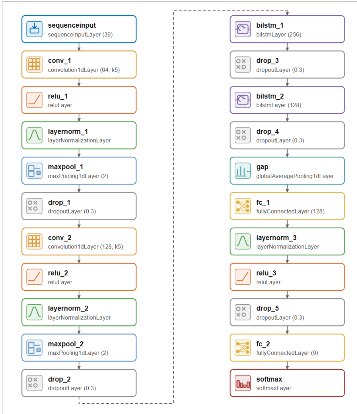
Figure 5. CNN+BiLSTM model architecture.
